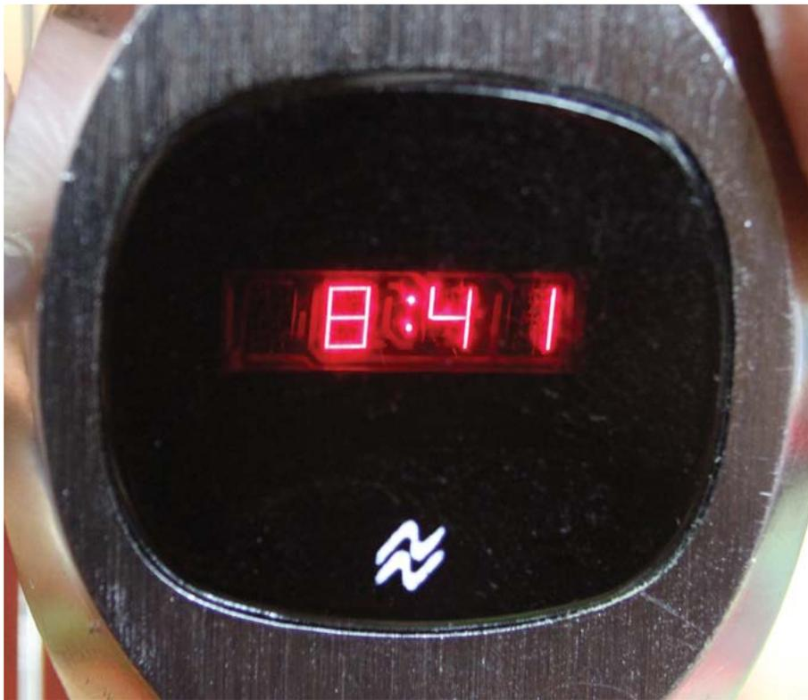
**Figure 8, left.** National semiconductor-light-emitting diode (LED) illuminated red digits, metal tonneau case with a push button that activates the digital display, ca. 1970s.
