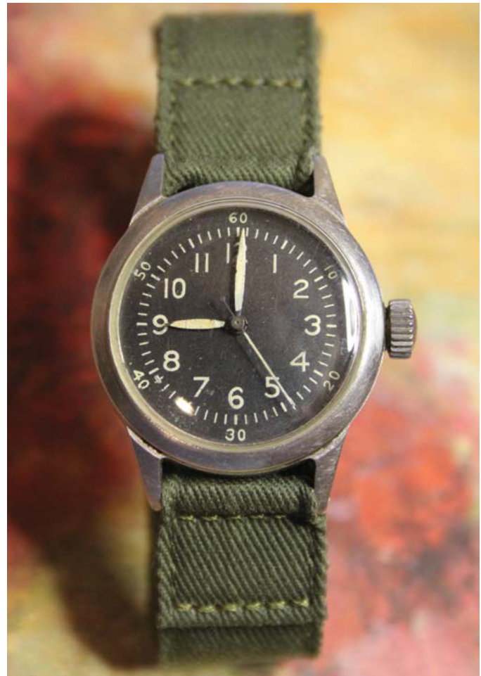
Figure 1. U.S.-made World War II military wristwatch with a 16-jewel movement and hack set functionality by Waltham, ca. 1944.
